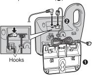
3 Mount the unit on a wall then slide down to secure in place.
