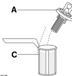
3. Turn the handle about  $\frac{1}{4}$  a turn anticlockwise and remove.
