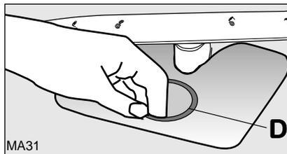
7. Put the flat filter (D) back in the base of the washing compartment.
