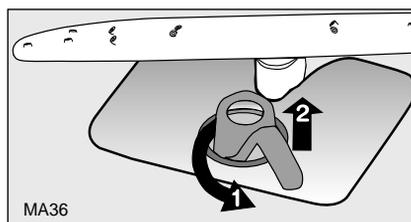
4. Take hold of the coarse/fine filter (A/B) by the handle with the hole and remove from the microfilter (C).
