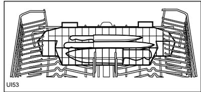
Forks and spoons should be placed in the removable cutlery basket with the handles facing downwards and the knives with their handles facing upwards.
