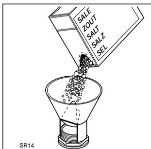
The salt container will require topping up periodically. You are reminded of this by the salt indicator light on the control panel which comes on when the salt has finished.
