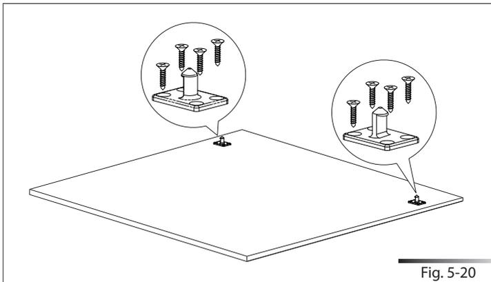
Drill holes for the panel handle using a drill with a suitable bit. Use the screwdriver to secure the door handle before hooking the panel to the dishwasher (see fig. 5-21).
