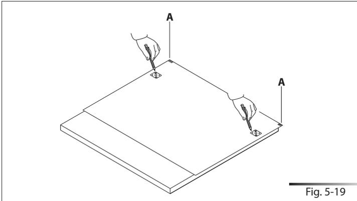
Use the screwdriver to secure the door hooks with the 8 supplied screws (see fig. 5-20) at the marked reference points.
