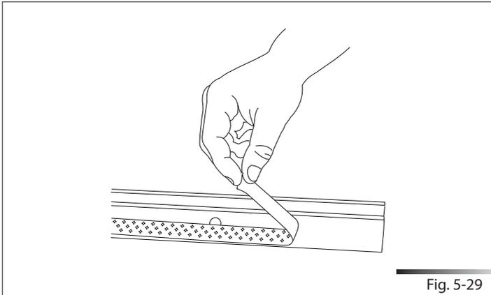
Fix the gasket to the dishwasher, inserting it in the seat on the sides towards the front (see fig. 5-30), and making sure that the long side of the gasket, the one with the hole for inserting the screw, is attached to the outside of the dishwasher; the hole in the long side must match the hole in the dishwasher (see ref. A fig. 5-31). Make sure the gasket adheres perfectly to the dishwasher.
