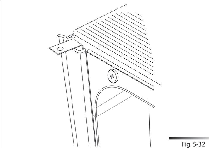
Tighten the supplied screws with a screwdriver; this operation definitively fixes the dishwasher to the adjacent units; cover the side holes using the supplied plugs (ref. A fig. 5-33).
