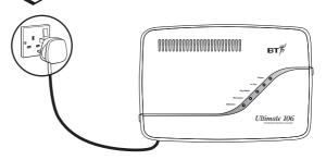
Connect the 3-pin plug into the mains socket and switch the power on. The POWER light comes on.
