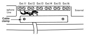
Replace the cable clamp when finished.
