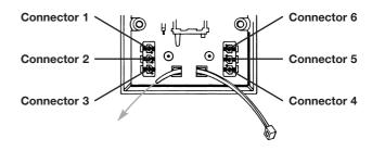
Thread the plastic wire grip through the socket (as shown above).
