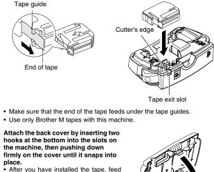
After you have installed the tape, feed the tape (  $_{\text{Shift}}$  +  $_{\text{Print}}$  ) once and then push in the tape cutter lever to cut
