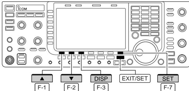
A total of 3 meter types are available in the IC-7700—Standard, Edgewise and Bar meters. Follow the instructions below for the meter type selection.
