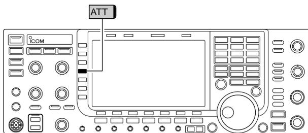
The attenuator prevents a desired signal from distortion when very strong signals are near the desired frequency or when very strong electromagnetic fields, such as from broadcasting stations near your location.
