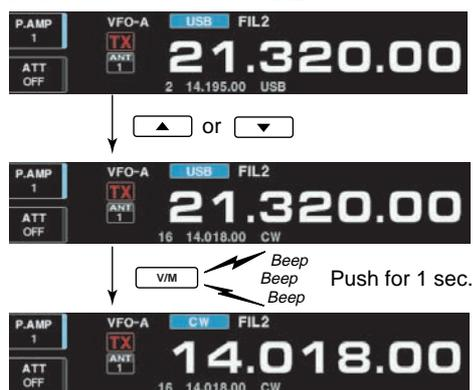
The frequency and operating mode in a memory channel can be transferred to the VFO. Frequency transferring can be performed in either VFO mode or memory mode.
