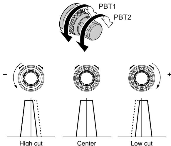
62 PBT CLEAR SWITCH [PBT-CLR] (p. 5-12)
