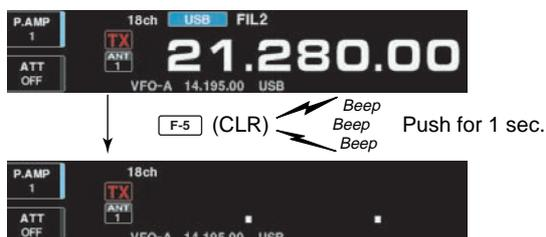
Any unused memory channels can be cleared. The cleared memory channels become blank channels.
