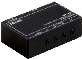
For remote transceiver control using a PC. You can change frequencies, operating mode, memory channels, etc. (software is not included)
