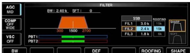
The IC-7700 has 3, 6 and 15 kHz roofing filters at the 1st IF frequency. The roofing filter provides interference reduction from nearby strong signals.
