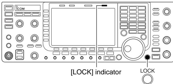
The dial lock function prevents frequency changes by accidental movement of the tuning dial. The lock function electronically locks the dial.
