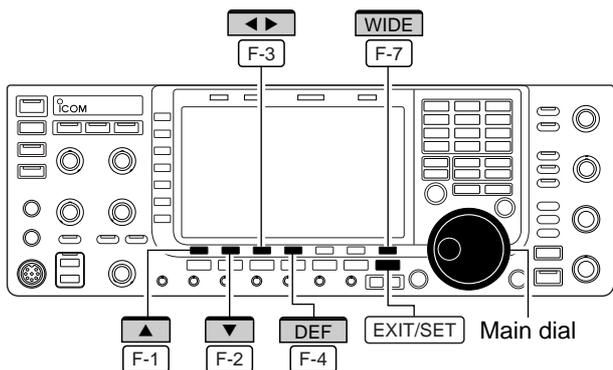
This set mode is used to set the waveform color, sweeping speed, scope range for fixed mode, etc.
