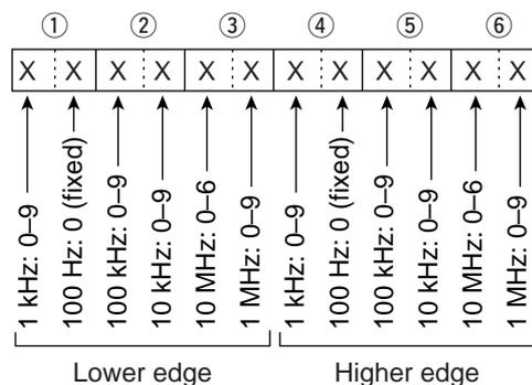
◆ Data mode with filter width setting
