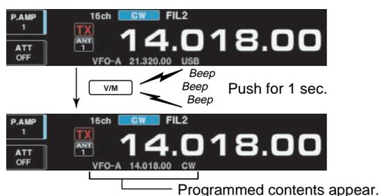
This is useful for transferring frequency and operating mode while operating in memory mode.
