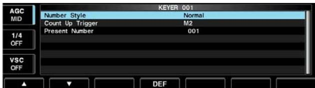
This menu is used to set the contest (serial) number and count-up trigger, etc.
