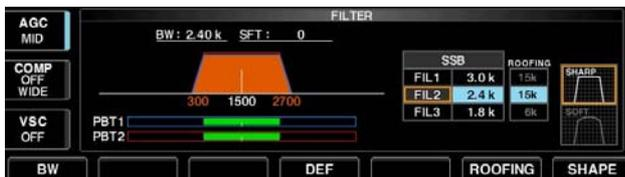
① Push and hold **[FILTER]** for 1 sec. to enter filter set screen.
