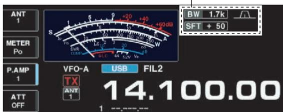
PBT (Passband Tuning) electronically narrows the IF passband width by shifting the IF frequency slightly outside of the IF filter passband to reject interference. The IC-7700 uses DSP for the PBT function. Moving both [TWIN-PBT] controls to the same position shifts the IF for both high and low frequencies.
