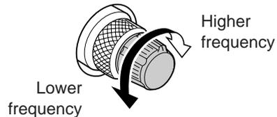
**65 MANUAL NOTCH FILTER CONTROL [NOTCH]**
