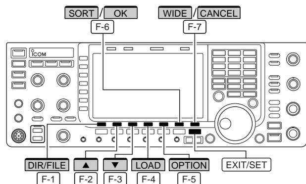
By loading the saved setting file from the USB-Memory, you can easily set up another IC-7700—several operators settings can easily be applied to one IC-7700.
