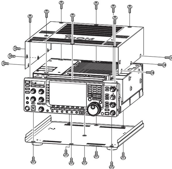
**CAUTION!** DISCONNECT the AC power cable from the transceiver before performing any work on the transceiver. Otherwise, there is danger of electric shock and/or equipment damage.
