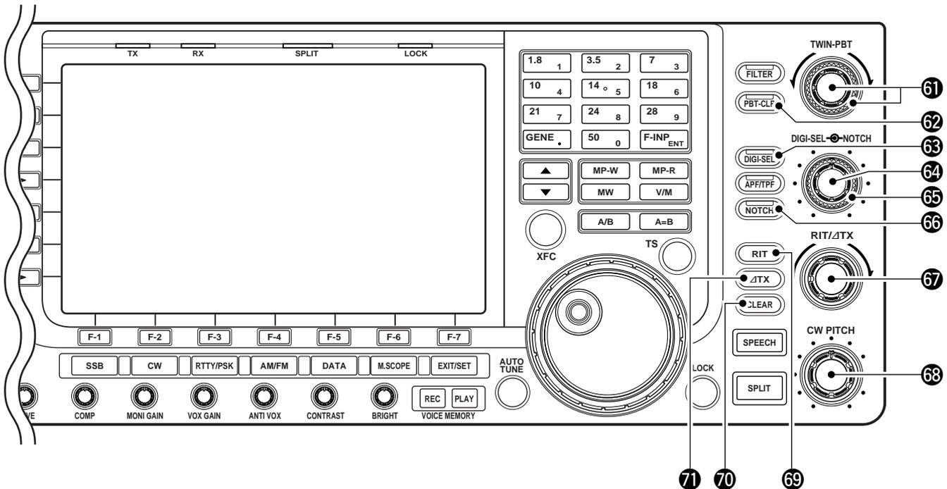
61 PASSBAND TUNING CONTROLS [TWIN-PBT]
