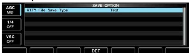
The contents of the RTTY memory and received signal can be saved into the USB-Memory.
