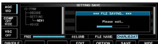
Memory channel contents, set mode settings, etc. can be saved into the USB-Memory for backup.
