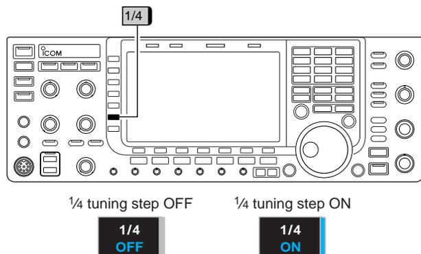
When operating in SSB data, CW, RTTY or PSK, the 1/4 tuning function is available. Dial rotation is reduced to 1/4 of normal speed when the 1/4 tuning function is ON for finer tuning control.
