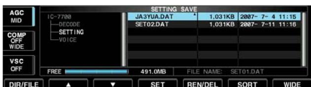
The file name, saved in the USB-Memory, can be re-named from the transceiver as desired.
