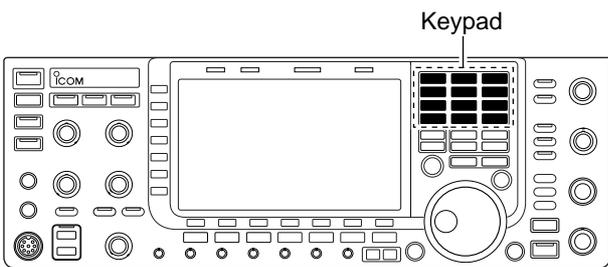
The transceiver has a keypad for direct frequency entry as described below.
