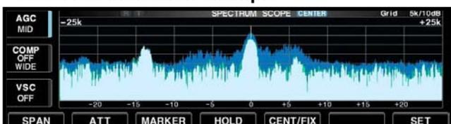
This DSP-based spectrum scope allows you to display the conditions on the selected band, as well as relative strengths of signals. The IC-7700 has two modes for the spectrum indication— one is center mode, and another one is fixed mode.
