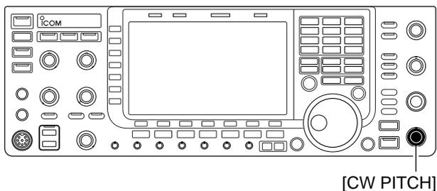
The received CW audio pitch and CW side tone can be adjusted to suit your preference (from 300 to 900 Hz in 5 Hz steps). This does not change the operating frequency.
