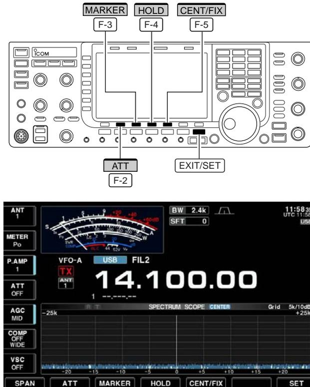
Displays signals within the specified frequency range. The selected frequency band conditions can be observed at a glance when using this mode.
