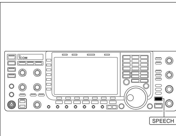
The IC-7700 has built-in voice synthesizer to announce the frequency, mode, etc. (S-meter level can also be announced—p. 12-15) in clear, electronically-generated voice, in English (or Japanese).
