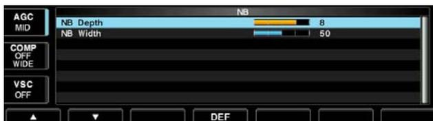
To deal with various type of noises, attenuation level and noise blank time can be set in NB set mode.
