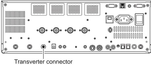
When 2 to 13.8 V is applied to pin 6 of [ACC 2], the [X-VERTER] connector is activated for transverter operation and the antenna connectors do not receive or transmit any signals.
