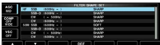
The type of DSP filter shape for SSB, SSB data and CW can be selected independently from soft and sharp.
