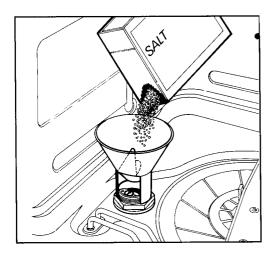
When this has been done, all you have to do is to periodically add salt to the container. You are reminded of this by a green refill indicator on the cap of the water softener.
