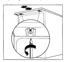
You can move the worktop forward or backward by 25 mm in order to align the machine with the other kitchen units.
