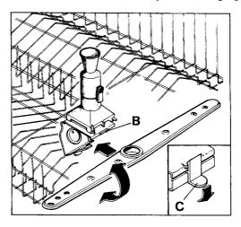
To do so, unhook the upper spray arm from the central support B by pressing the clip C and refit it in a reverse position (holes on the bottom). In this way the wash efficiency is improved, as the bottom basket is sprayed by both arms.
