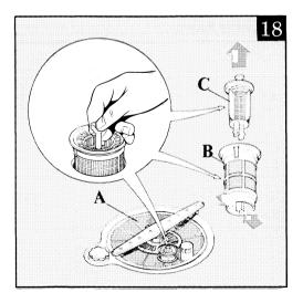
There are three filters (see fig. 18 below), one large circular fine-mesh tilter (A) and two small cone-shaped ones (B & C).
