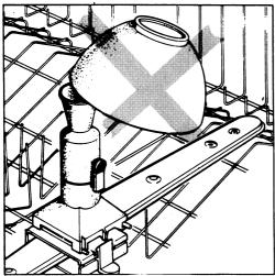
Before closing the door, ensure that the spray arms can rotate freely.
