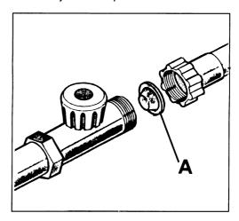
**Caution:** the retaining ring must be correctly fitted to avoid water leaks.
