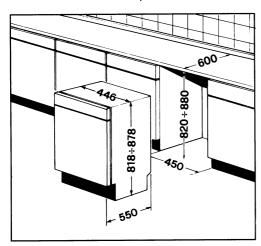
The recess ceiling may be anywhere between 820 and 880 mm from the floor inasmuch as the dishwasher incorporates levelling feet adjustable over a wide range (max 60 mm).
