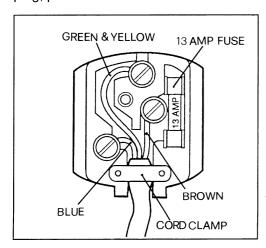
Connect the Green and Yellow (earth) wire to the terminal in the plug which is marked with the letter «E» or the earth symbol ⊕, or coloured green and yellow.
