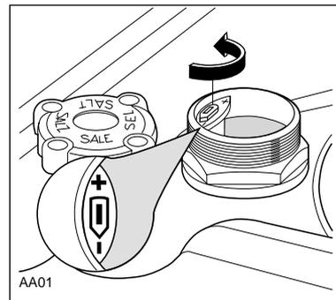
**i** If your water is level 1 it is already soft and therefore there is no need to use salt. In this case adjust the water softener on level 1 without using salt.
