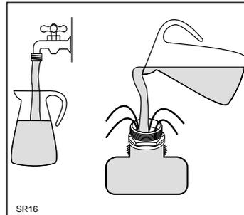
2. Pour 1 litre of water inside the container (this is necessary only before filling with salt for the first time).
