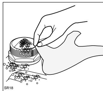
4. Remove any trace of salt on the screw thread or on the gasket.
