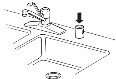
The drain air gap is usually located on top of the sink or countertop near the dishwasher. To order a drain air gap contact your local dealer, or in the U.S.A., call the Customer Interaction Center and ask for Part Number 300096.
