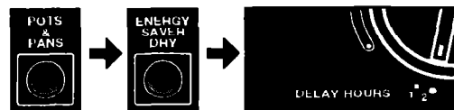
Example for 2-hour delayed Pots & Pans cycle with Energy Saver Dry option
