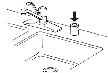
The drain air gap is usually located on top of the sink or countertop near the dishwasher. To order a drain air gap contact your local dealer, or in the U.S.A., call the Consumer Assistance Center at 1-800-253-1301 and ask for Part Number 300096.
