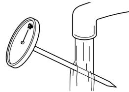
3. If the water temperature at the faucet is below 120°F (49°C), have a qualified person raise the water heater's thermostat setting.
