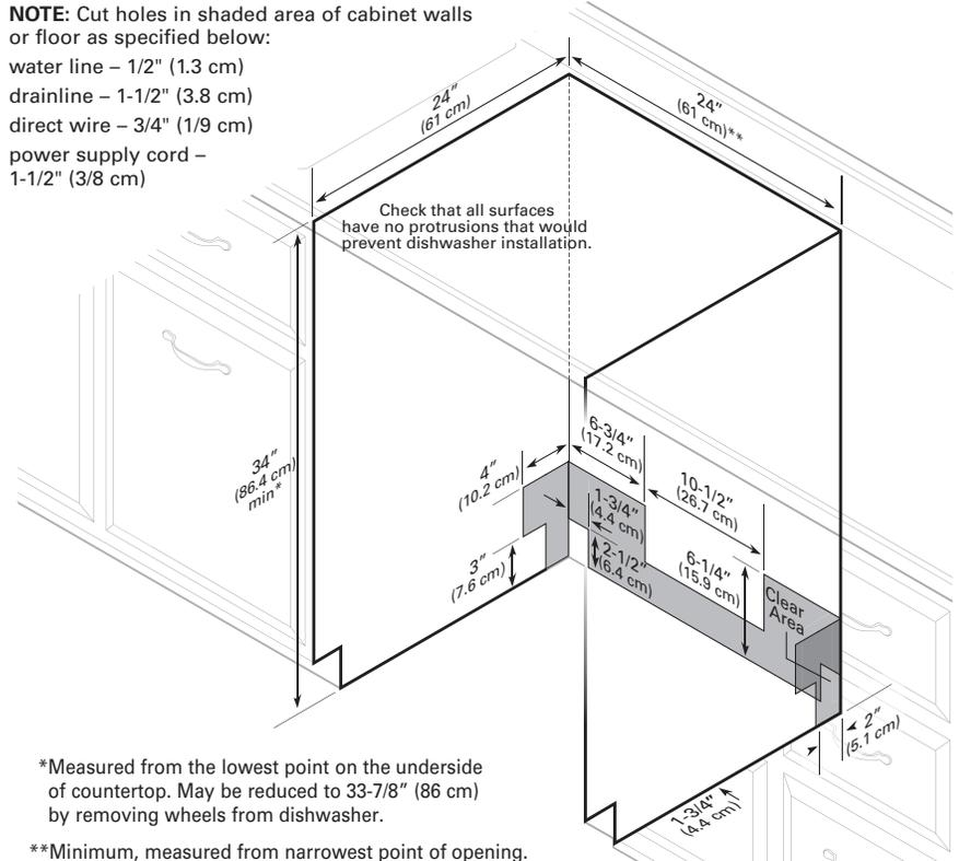
\*Measured from the lowest point on the underside of countertop. May be reduced to 33-7/8" (86 cm) by removing wheels from dishwasher.
