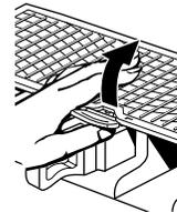
**NOTE:** Be sure the cover is completely latched before pulling out the bottom rack and before closing the dishwasher door.
