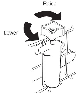
2. With the other hand, turn the knob clockwise to raise a side of the rack.
