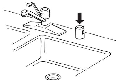
The drain air gap is usually located on top of the sink or countertop near the dishwasher. To order a drain air gap, contact your local dealer; or in the U.S.A., call the Customer Interaction Center and ask for Part Number 300096.
