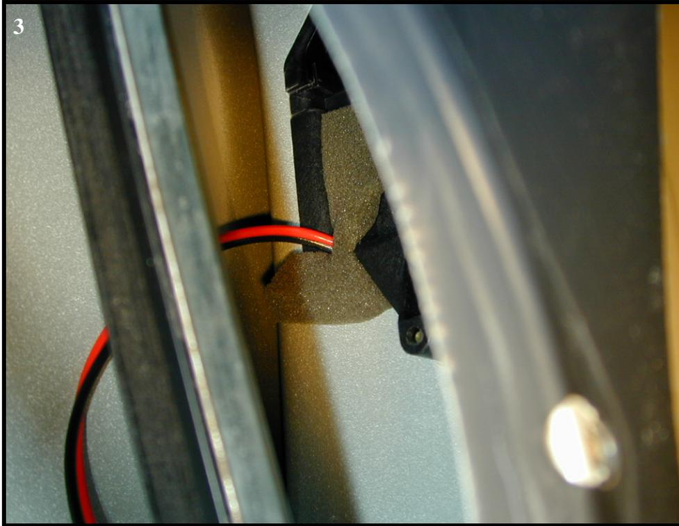
3. Guide the wire harness down into the door and bolt the mirror housing on the door. On the inside of the door there are two small holes at the bottom of where the plastic canister base is attached. The holes may be hidden behind foam insulation. Guide the wire harness through the left hole and out of the door.
