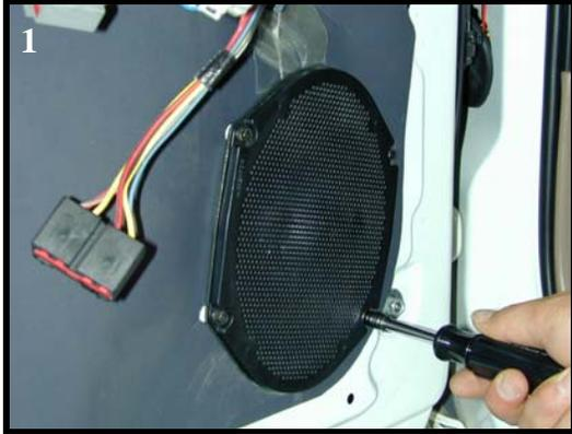
1. Remove the screws around the door speaker.
