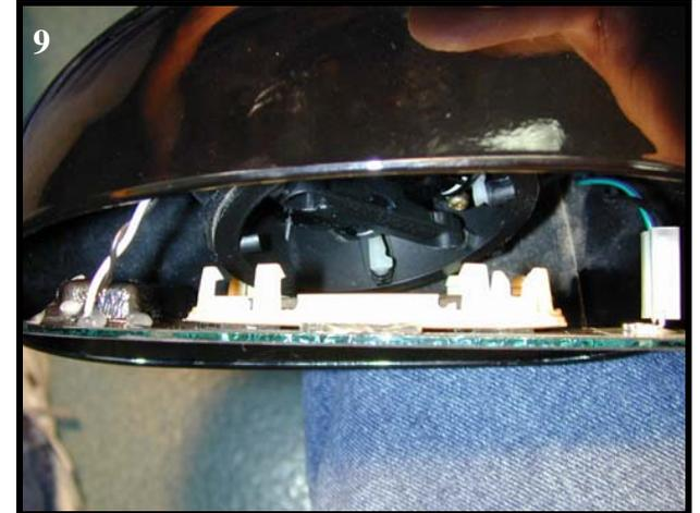
Tuck the wires toward the back of the mirror housing. Align the *Signal*® mirror over the center hub of the mirror housing and firmly press the mirror into the housing until it snaps into position.
