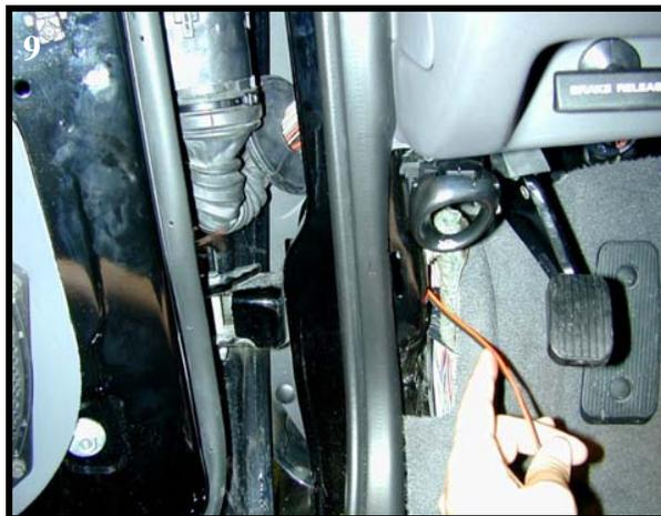
5. Pull the rubber boot out from the door frame.
