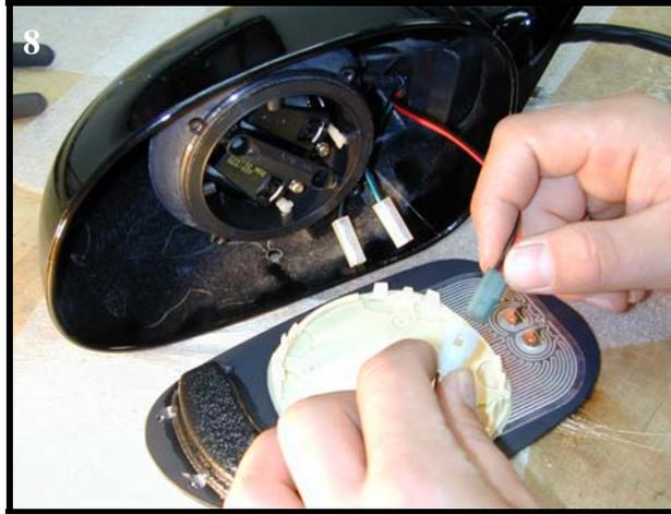
Cut a slot in the foam disc just large enough to accommodate the anti-rotation prongs on the motor adaptor (on the *Signal*® mirror). Place the foam disc on the back of the *Signal*® mirror. If your mirrors have the heater option, connect the heater mirrors at this time. Connect the *Signal*® mirror mating connector to the *Signal*® mirror wire harness.
