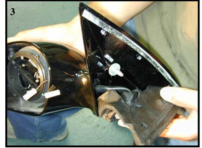
3 Carefully peel back the foam insulation on the mirror housing sail.
