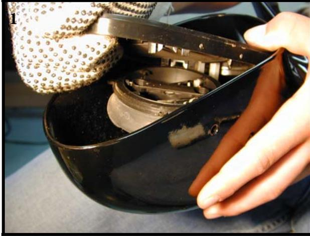
1 While using sturdy gloves, position your fingers behind the outboard edge of the mirror. Pull back on the mirror to dislodge it from the center hub and remove the mirror from the housing.
