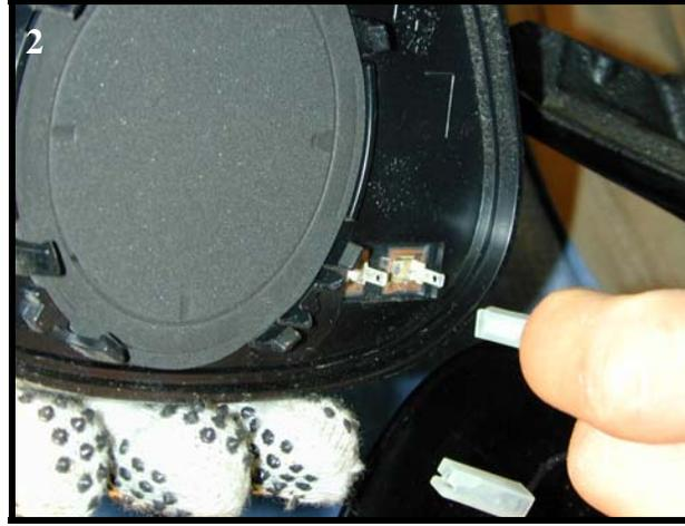
2 If your mirrors have the heater option, disconnect the heater wires at this time. Carefully remove the foam disc from the back of the mirror and set it aside.
