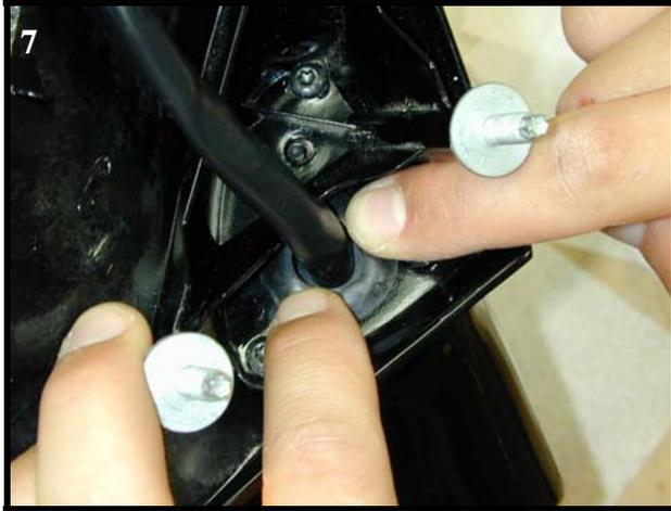
Pull the rubber grommet back out from the mirror housing and reposition.
