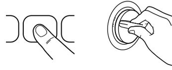
3. Turn the Cycle Control knob clockwise to the number of hours you want the dishwasher to delay the start.
