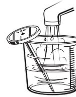
3. Check the temperature on the thermometer as the water is running into the cup.
