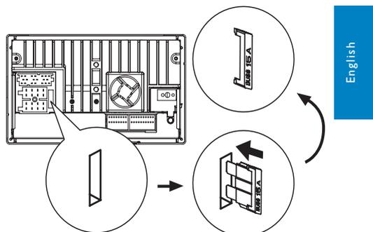
If the fuse gets damaged immediately after it has been replaced, there may be an internal malfunction. In such case, consult your Philips dealer.
