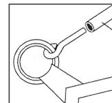
**K)** Take the Eave Pole (EPOL-26BK) and put into yellow taped opening on all six hubs.
