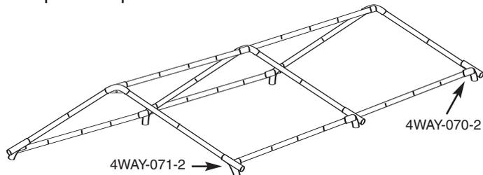
**H)** Position the tent body underneath the roof assembly. Hook S-hooks on tent body roof to the holes in each corresponding hub. Also connect quick clips to the poles.
