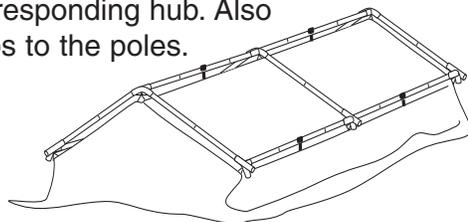
**I)** The Corner Leg Poles (LPSA-168BK) will insert into the hubs on all four corners with the green tape.
