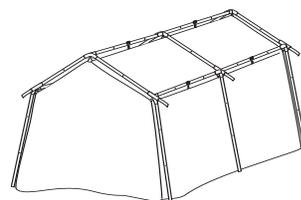
**J)** Take the Center Leg Poles (LPCA-168BK) and put into purple opening on hubs in the center. Insert pins into pole ends.
