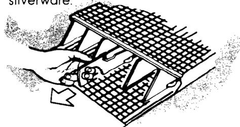
**To remove the basket**, slide it toward the top of the door – by the handle. Lift it off the holding buttons. Replace it in reverse order.
