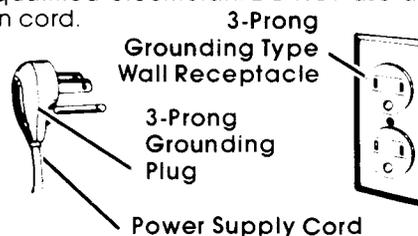
**DO NOT, UNDER ANY CIRCUMSTANCES, REMOVE THE POWER SUPPLY CORD GROUND PRONG.**
