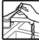
2. Hold a candy or meat thermometer in the running stream of water. If the water temperature at the faucet is below 120°F (49°C), have a qualified person raise the water heater's thermostat setting.
