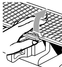
**NOTE:** Be sure the cover is completely latched before pulling out the bottom rack and before closing the dishwasher door.
