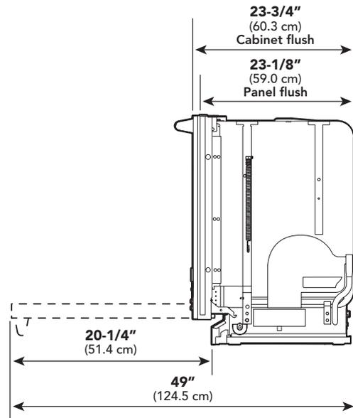
**Note:** If the dishwasher is installed in a corner, there must be a minimum clearance of 2" (5.1 cm) from the side wall so the door can open.
