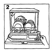
2. Load the dishwasher. (See page 16: "How to load the dishwasher"). Pour approx 15 g detergent into the detergent compartment inside the door. If the dishes are normally or heavely soiled add an extra 5 g anywhere on the inside of the door. Close the door.
