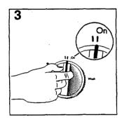
Plug in the dishwasher Start the dishwasher by turning the programme knob to the "On" position.
