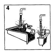
4. At the end of the programme switch off the dishwasher by turning the programme knob until the programme knob is in vertical position in line with the thick market on the facia. When the crockery has been removed, clean the filters and turn off the water supply.
