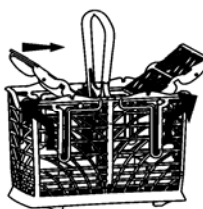
Movement required to extract the inserts
