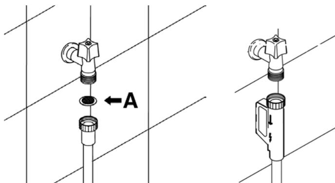
The dishwasher can also be connected to a hot water supply **not exceeding 60°C**. Supplying the appliance with hot water cuts down the washing time by approximately 20 minutes, but slightly reduces its effectiveness. Make the connection to the domestic hot water supply using the same procedure described for connecting to the cold water supply.
