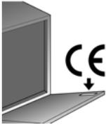
THE NAME PLATE FEATURING THE TECHNICAL DATA, SERIAL NUMBER AND MARKINGS IS VISIBLY POSITIONED ON THE INNER EDGE OF THE DOOR. **THE NAME PLATE ON THE INNER EDGE OF THE DOOR MUST NEVER BE REMOVED.**
