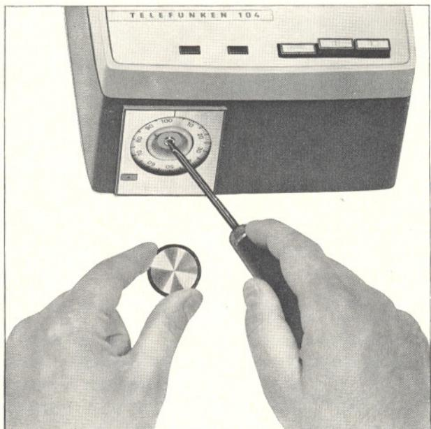
1. The counter ensures that only the preset number of telephone calls are accepted. This is very important as more calls may come in than recording tape capacity is available on the tape recorder. The recording tape capacity depends on the length of the tape available and the speed chosen on the tape recorder.
