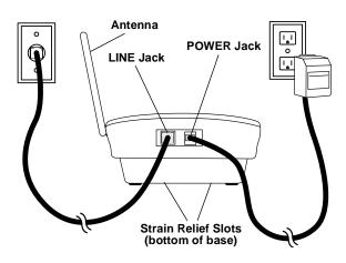
**1** Plug one end of the supplied long modular cord into the **LINE** jack on the back of the base.
