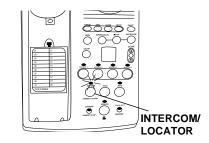
a longer time, hold down **INTERCOM/LOCATOR** for about 4 seconds. The handset beeps for about 3 minutes.
