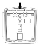
**3** Plug one end of the supplied short modular cord (or long modular cord if mounting directly on the wall) into the **LINE** jack and the supplied AC adapter's barrel plug into the **POWER** jack on the back of the base.
