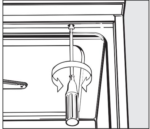
■ Remove the fixing screws on the left and right hand sides using a cross slotted screwdriver.
