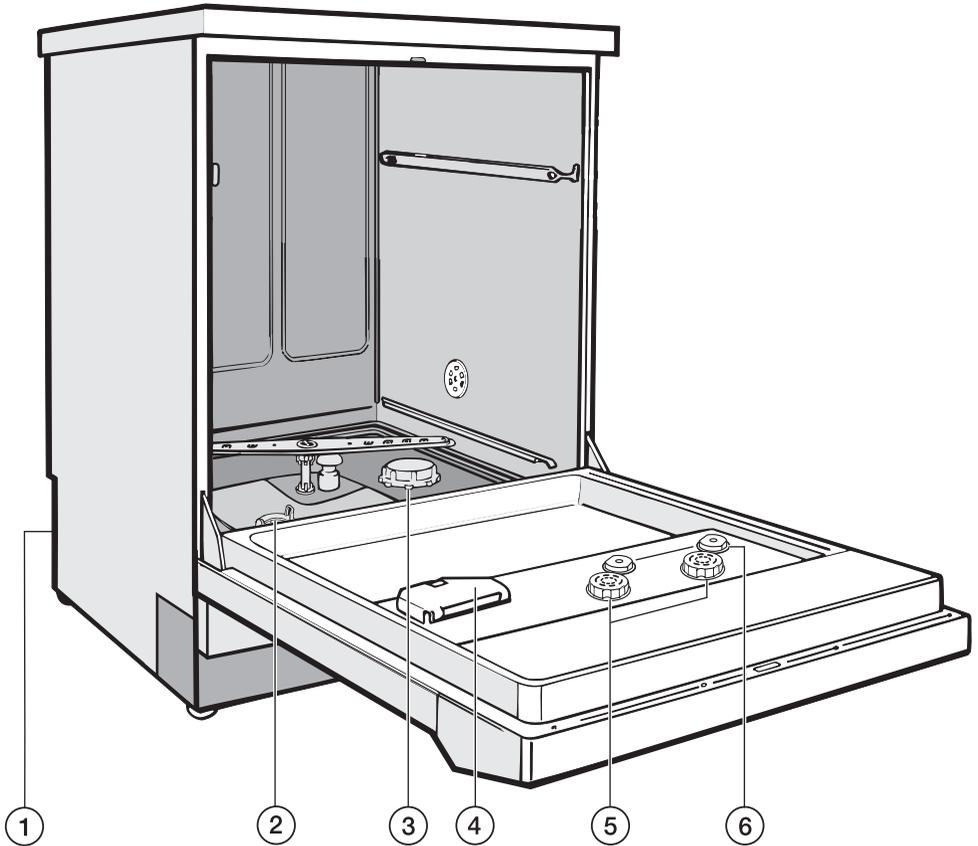
① Connections for optional DOS module dispenser pump for liquid cleaning agent - at the back of the machine -
