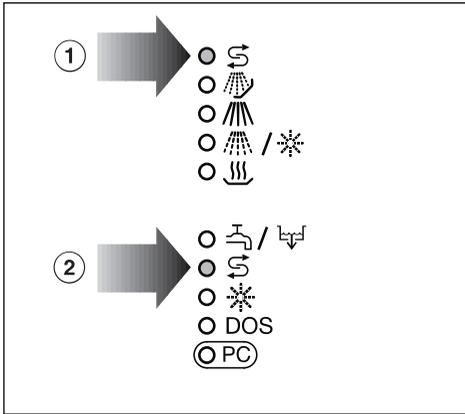
When the salt reservoir is empty the S indicator light ② comes on to remind you to fill the reservoir.
