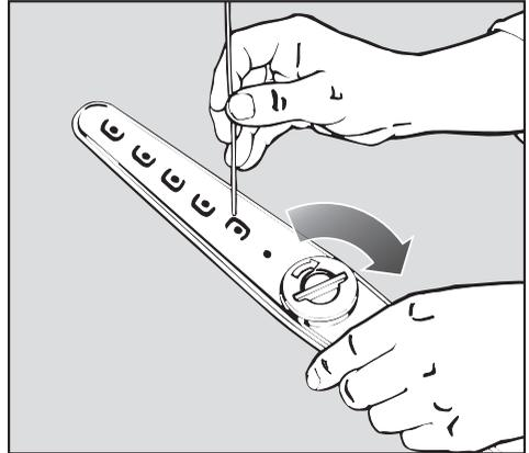
Particles in the lower spray arm are easier to rinse out if the cap is first opened.
