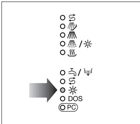
If the \* Add rinsing agent indicator light on the control panel comes on, the rinsing agent reservoir must be refilled.
