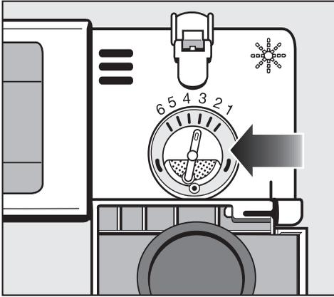
The dosage adjuster in the opening has settings from 1 to 6 (1-6 ml). It is set to 3 (3 ml) at the factory as the recommended dosage for **rinsing agent**.
