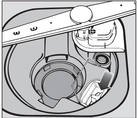
The drain pump is beneath the non-return valve (see arrow).
