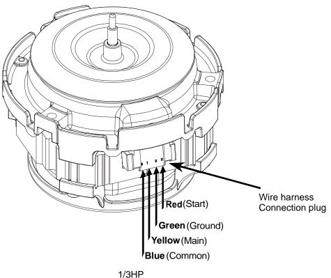
120V/60hz, 3.2 amps, 3250 RPM
