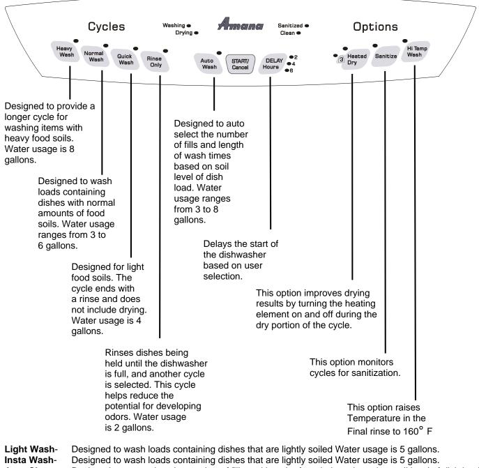
Auto Clean- Designed to auto select the number of fills and length of wash times based on soil level of dish load. Water usage ranges from 3 to 8 gallons.
