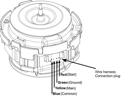
1/3HP 120V/60hz, 3.2 amps, 3250 RPM
