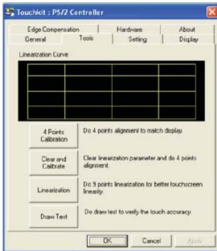
User can do calibration or draw test by pressing the function push buttons.
