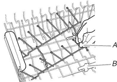
A. Lift removable insert wire to remove from holding clips.
