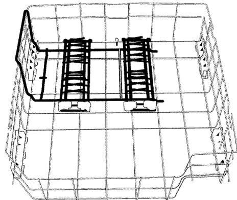
Removing this insert allows you to wash larger items such as large mixing bowls, stock pots, and roasters.
