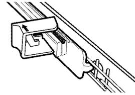
3. Place the back rack rollers on each side of the culinary tool rack into the track slots and roll the rack back into the tracks.
