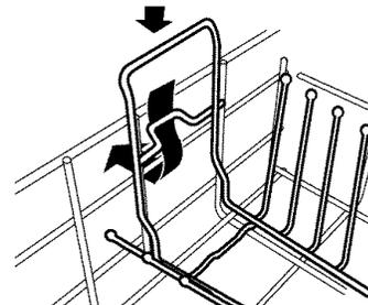
3. When center tab under handle locks in under the middle side rack wire, the insert is in place. (See illustration.)
