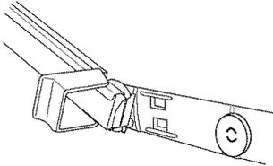
4. Insert front rack rollers on each side of the rack into the rack slots.
