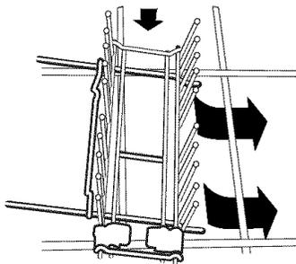
2. Push down on insert until handle fits against outer rack edge.
