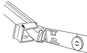
4. Insert front rack rollers on each side of the rack into the track slots and slide rack partly back into the dishwasher.
