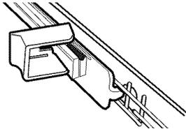
3. Place the back rack rollers on each side of the rack into the track slot and roll the rack back into the tracks.
