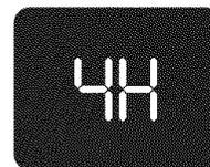
showing in the display. The 4 Hour Delay light will glow.
