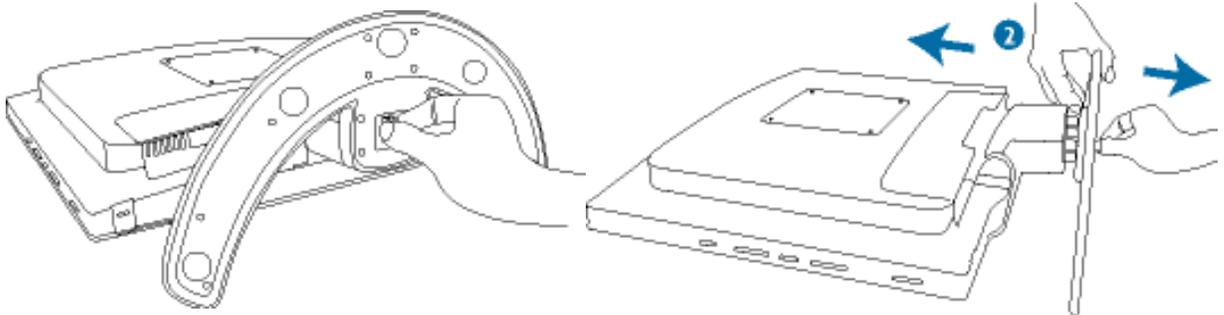
2) Press the release latches on the bottom of the base together and gently remove the attachment unit from the base.
