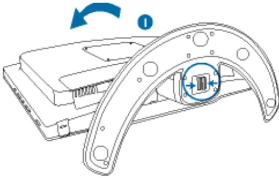
1) Place the monitor face down a smooth surface taking care to avoid scratching or damaging the screen.
