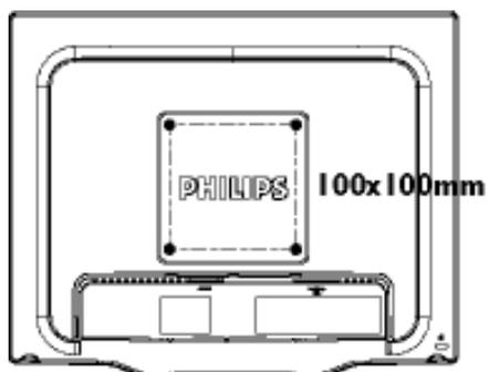
**Note:** This monitor is designed to work with a 100mm x 100mm VESA-compliant mounting interface.
