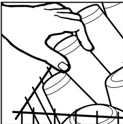
2. Spin the upper spray arm. It should turn freely. Check the lower spray arm also to make sure it turns freely.
