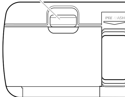
2. Fill the Main Wash section with detergent. The amount of detergent needed depends on the amount of food soil on the dishes and water hardness. See the detergent usage chart later in this section.
