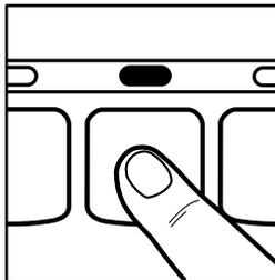
8. Press the Start pad. The cycle will begin (if Delay Hours has not been selected). **NOTE:** The dishwasher remembers the last cycle and option(s) that were completed. You only have to press the Start pad if you want to use the same cycle and option(s). However, if the last cycle you completed was Rinse Only, the dishwasher will run the Normal cycle if you press the Start pad.
