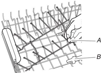
A. Lift removable insert wire to remove from holding clips.
