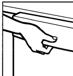
2. Spin the upper spray arm. It should turn freely. Check the lower spray arm also to make sure it turns freely.
