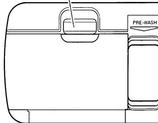
2. Fill the Main Wash section with detergent. The amount of detergent needed depends on the amount of food soil on the dishes and water hardness. See the detergent usage chart on page 14.
