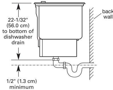
If the dishwasher drain exits through the back wall, the centerline of the drain must be a minimum of 1/2" (1.3 cm) below the dishwasher drain. This is required to completely drain the dishwasher tub so that no standing water remains in tub.
