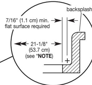
**IMPORTANT:** Corner radius dimensions specified must be used. If they are not, the dishwasher will not fit the opening.
