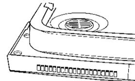
The vent closes during the cycle to lock sound in the dishwasher. After the cycle has finished, the vent remains closed until the dishes have cooled down. Between cycles, the vent stays open for air-flow, reducing the build-up of odors.
