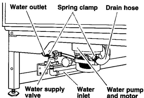
5. Remove the spring clamp from the water outlet and separate from the water supply valve; drain water into pan.
