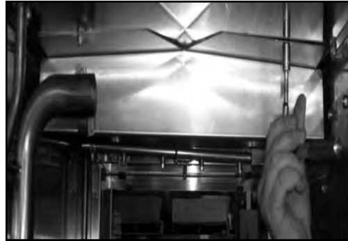
Removing and turning splash shield
