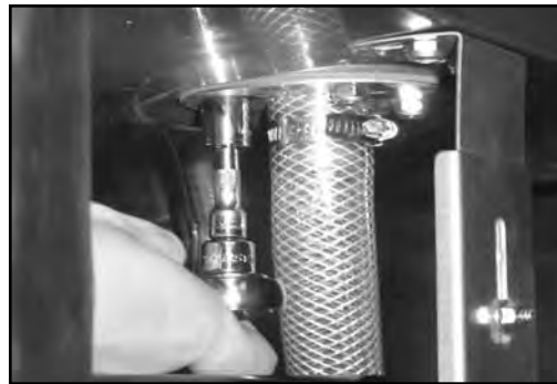
Removing the rinse drain weldment
