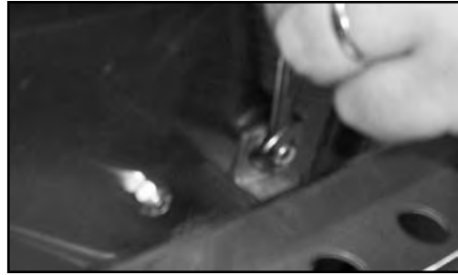
Removing the bracket nut
