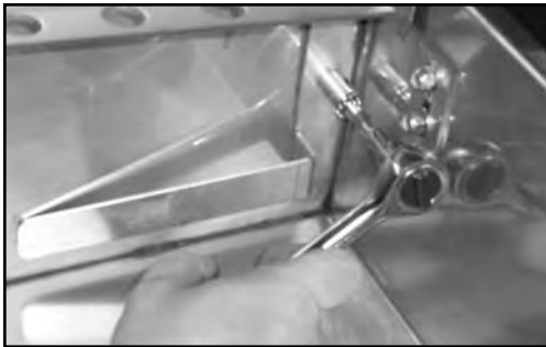
Removing a rinse tray guide bracket
