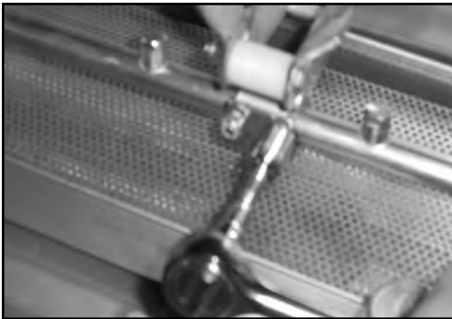
Removing the lower rinse arm support bracket
