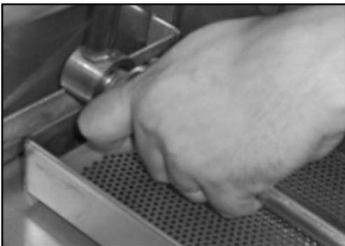
Unscrewing and removing the lower rinse arm
