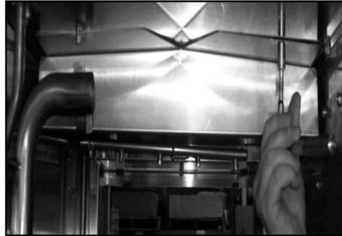
Removing and turning splash shield
