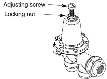
If the water level is too low or too high, check the incoming water pressure. It should be 20 ± 5 PSI. Too high of pressure results in too much water; too low of pressure results in too little water. To adjust the regulator, loosen the nut at the top, this will allow you to screw or unscrew the adjustment. With a screwdriver, turn the adjuster clockwise to increase pressure or counter clockwise to decrease it.
