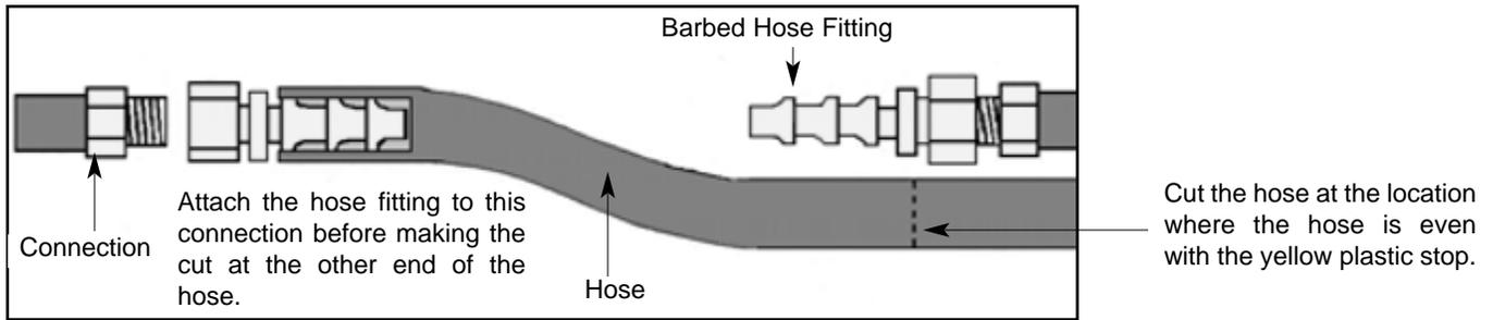
Due to the fact that each customer may have different requirements for the orientation of the gas booster heater relative to the main dishmachine, the hose lengths that connect the two units must be customized during each installation. The appropriate 3/4" hosing, fittings and gaskets have been provided.
