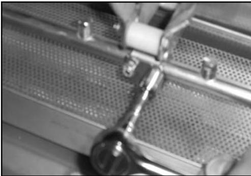
Removing the lower rinse arm support bracket
