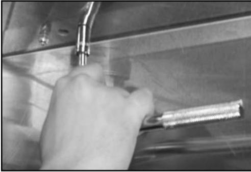
Removing the hole cover weldment
