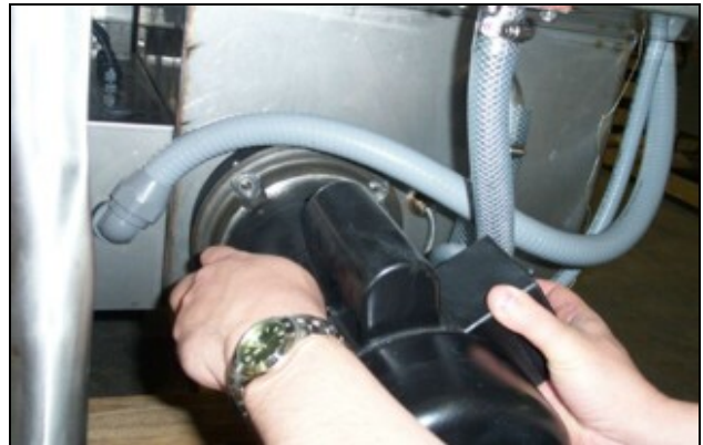
Remounting the wash motor assembly
