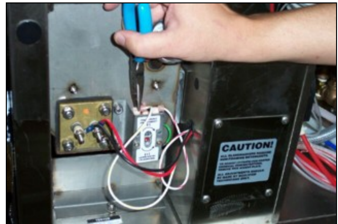
Removing the terminals.
