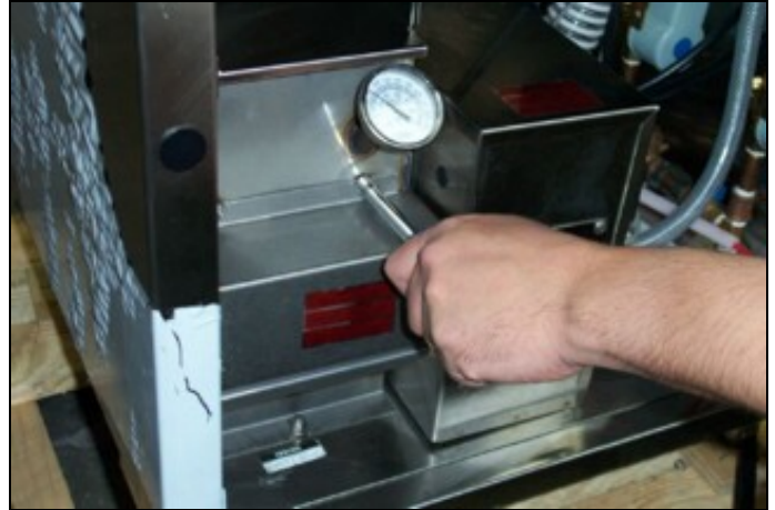
Removing the heater cover.
