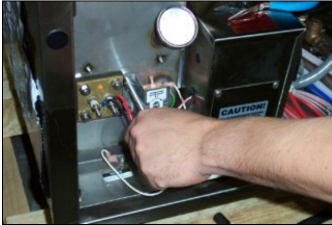
Removing the thermostat bracket mounting nuts.
