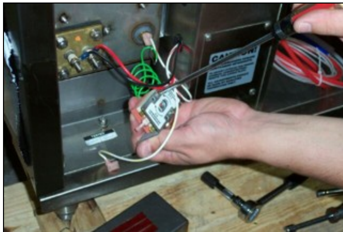
Separating the thermostat from the bracket.
