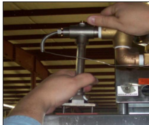
Lifting the rinse injector to make room
