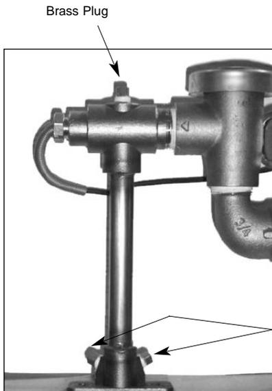
The 1/8" brass plugs on the incoming plumbing rinse injector may be removed to install sanitizer and rinse aid injection fittings.
