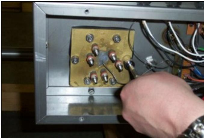
Removing the nuts and lockwashers
