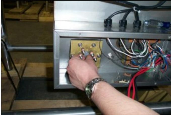
Removing silicone from thermostat well
