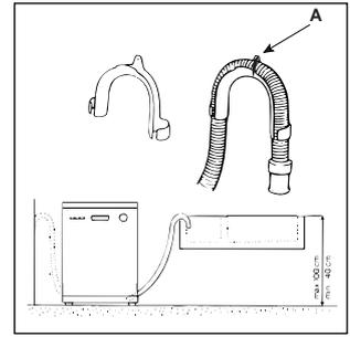
**Attention:** *The special plastic hose support must be solidly fastened to the wall to prevent the drain hose from moving and allowing water to spill outside the drain.*
